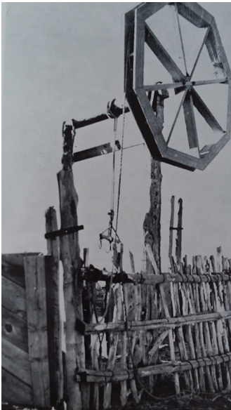
The photo above is of a homemade windlass for hanging meat on a desert ranch.
